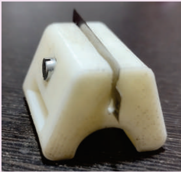
Fig. Prototype of modified loose flower plucker
